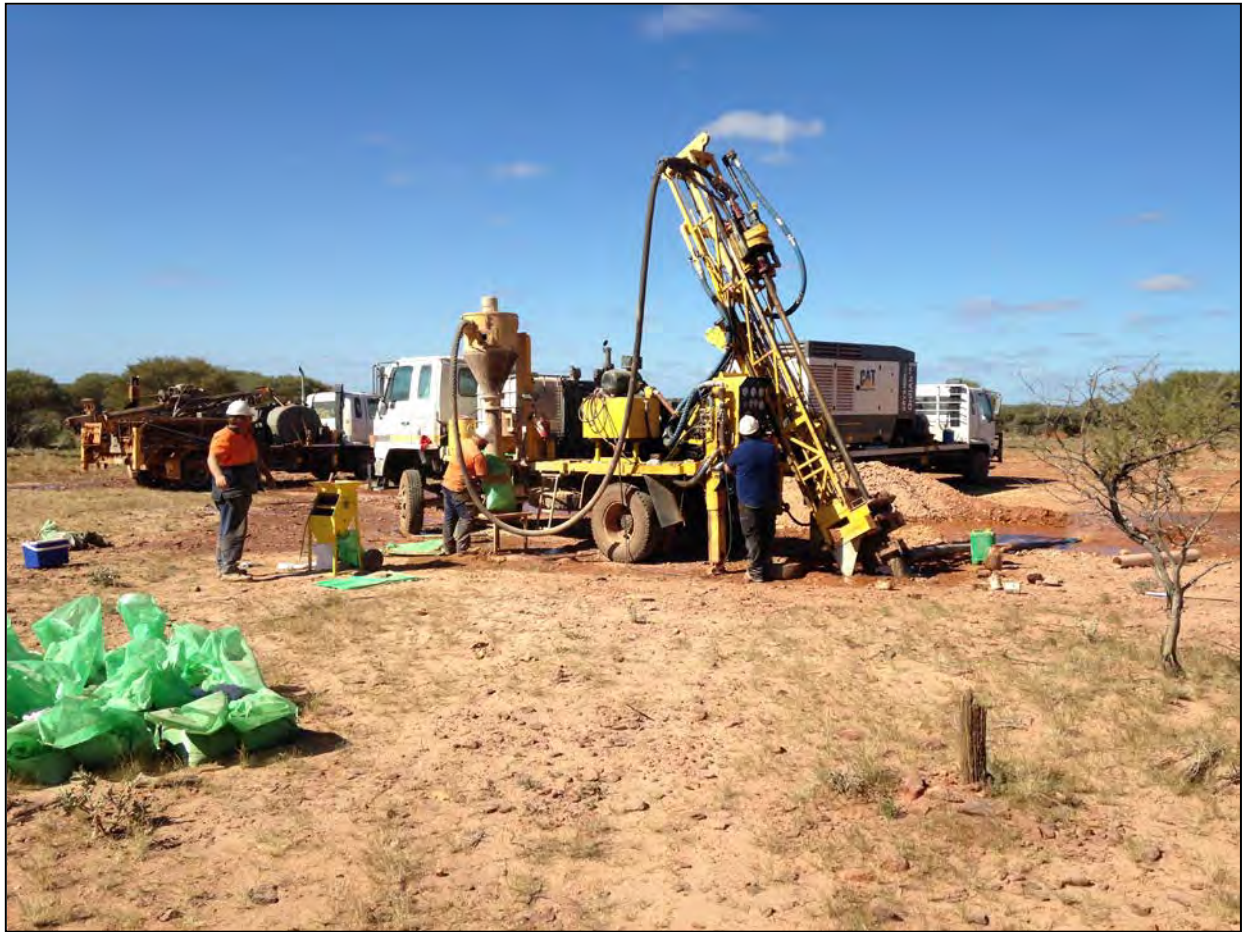
Figure 14 RC Drilling at Alliance on the eastern side of the open pit
