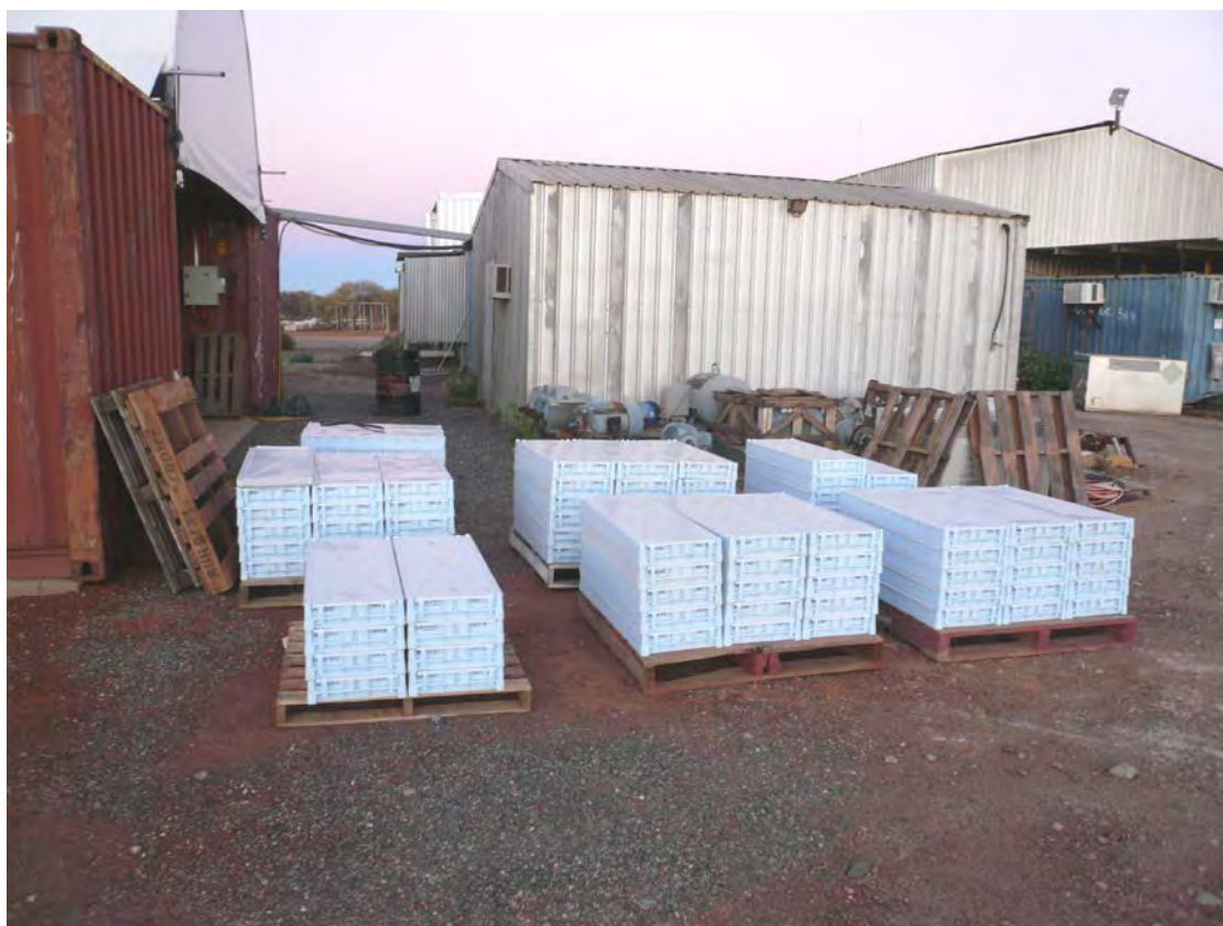
Figure 21 Diamond core trays containing whole PQ drill core stacked on wooden pallets awaiting securing with metal strapping prior to transport to ALS in Perth
