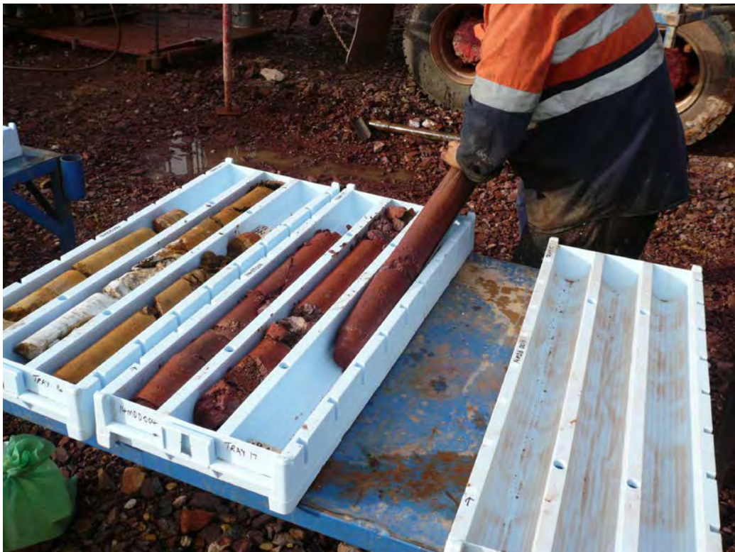
Figure 17 Hole 14MDD004 - PQ drill core inside the splits being pumped from the core tube
