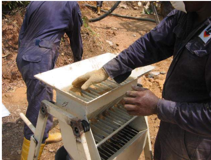
Figure 12.5 Pushing material through the splitter
