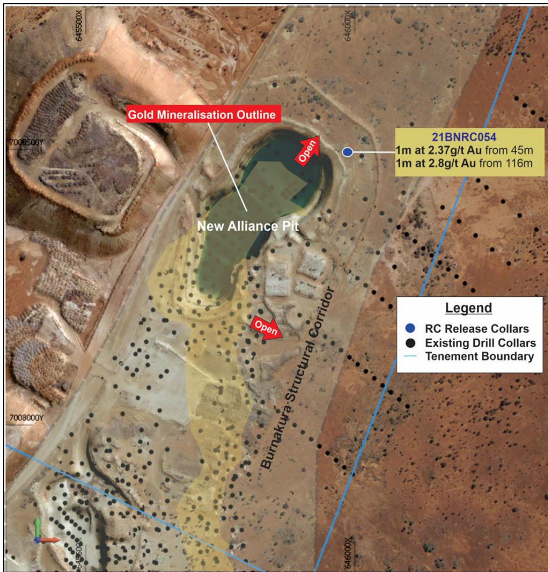
Figure 3: Phase 2 drilling completed for New Alliance target, showing anomalous RC intercepts previously reported.
