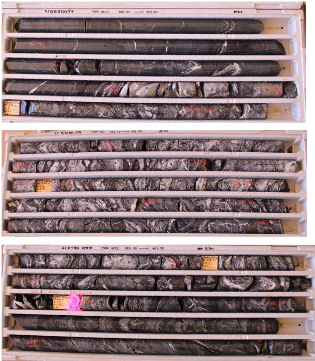
Figure 10: Picture of 21BNRD057 core showing intercepted mineralized package of highly deformed and altered sediments, mafic with minor fine-grained felsic rocks consistent with NOA Shear Zone.
