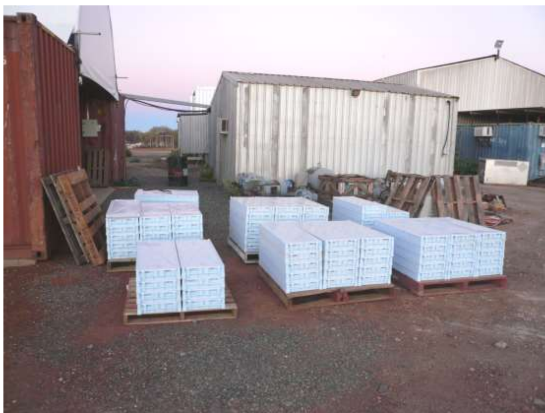
Figure 20 Diamond core trays containing whole PQ drill core stacked on wooden pallets awaiting securing with metal strapping prior to transport to ALS in Perth
