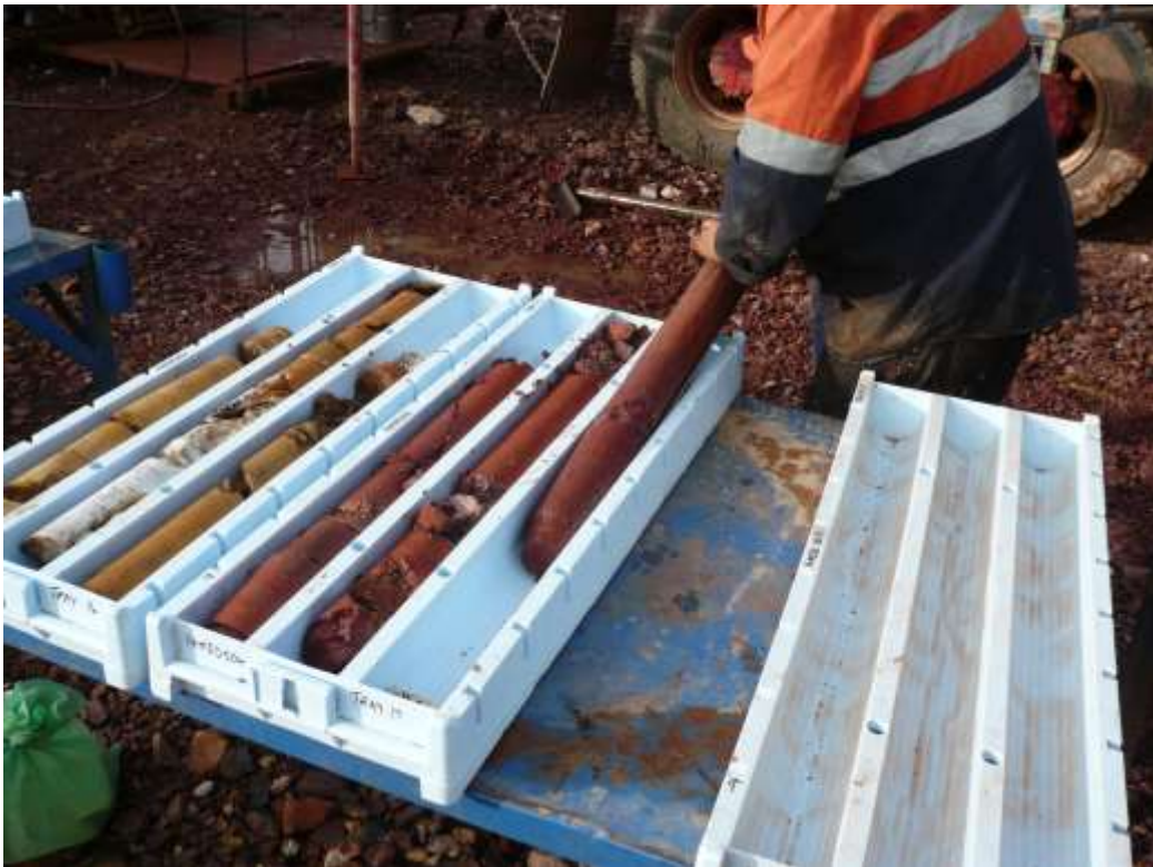
Figure 17 Hole 14MDD004 PQ drill core being transferred from the splits to core trays
