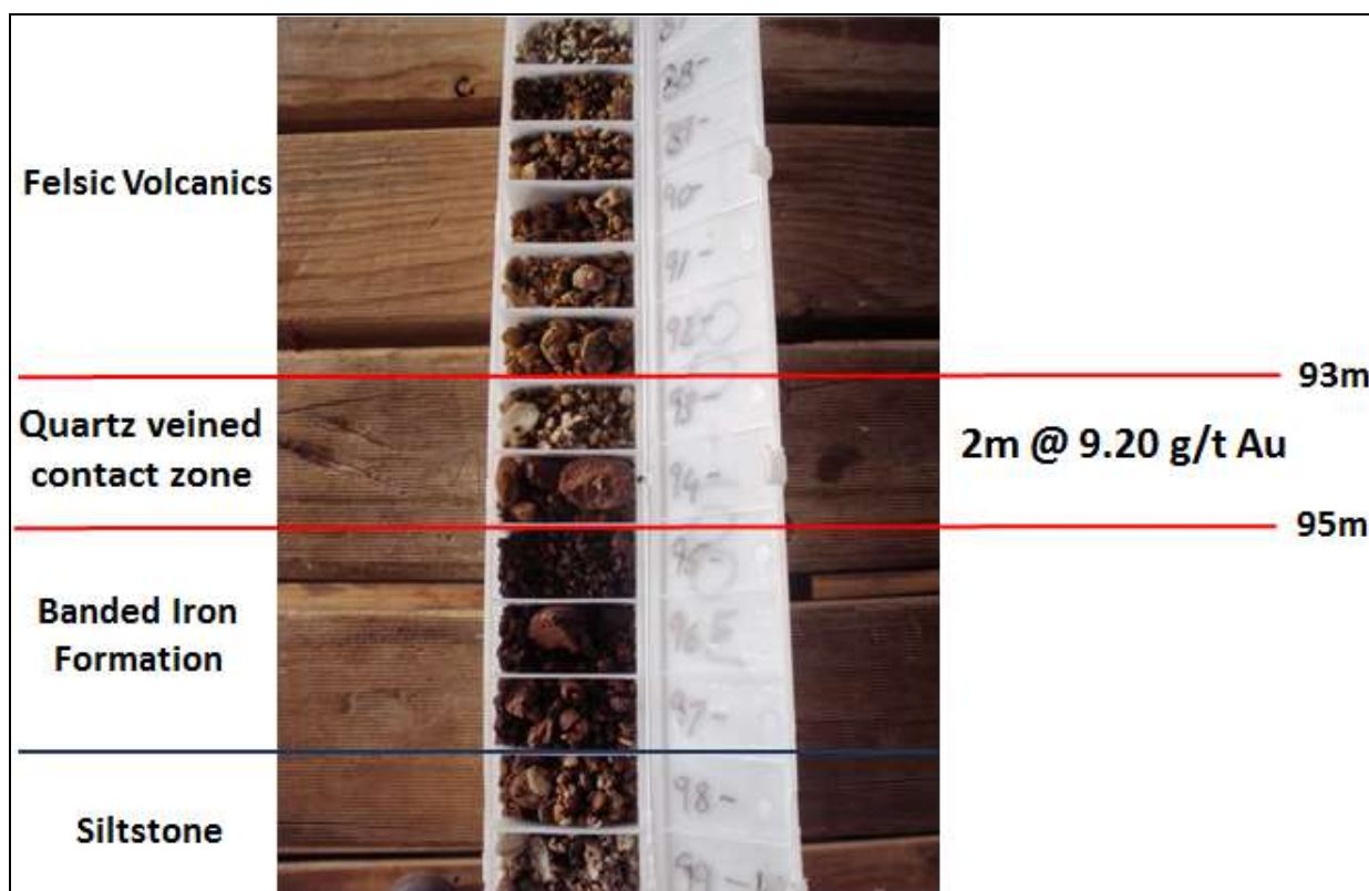
Figure 31 Independent Logging of 14MRC011 – 88m to 100m Downhole
