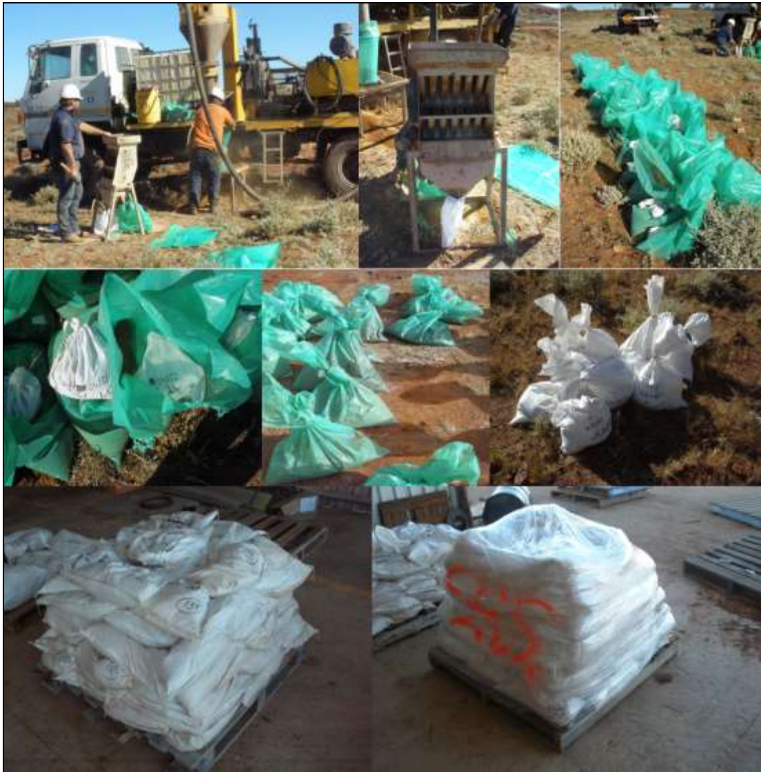
Figure 29 ANA – Drilling and Sampling Protocols from Drill Rig to Sample Dispatch
