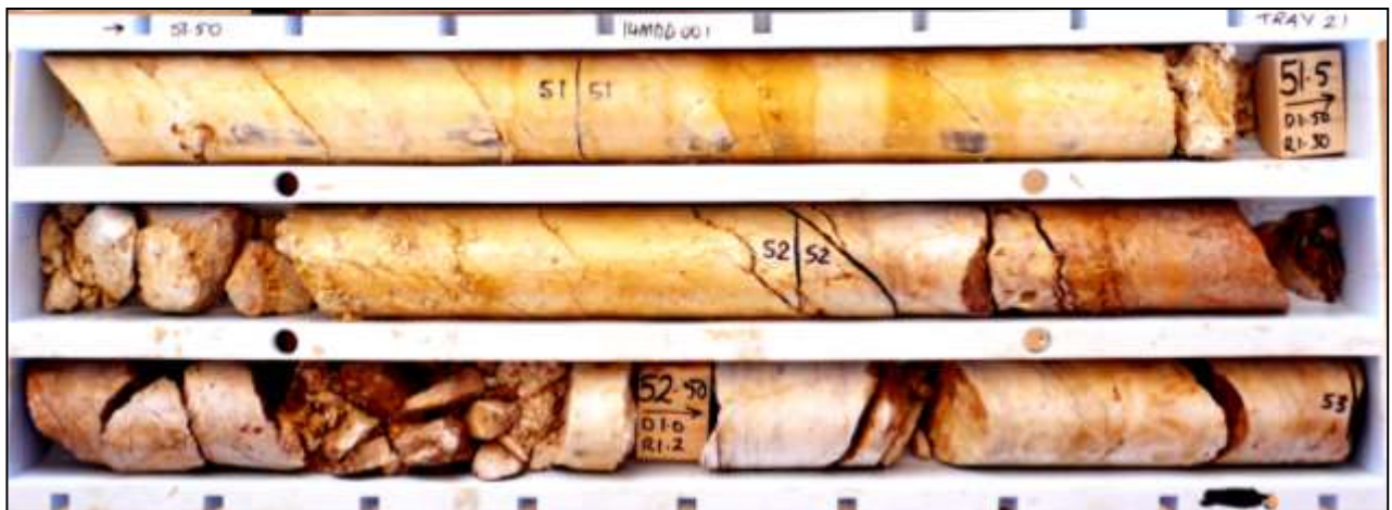
Figure 18 Hole 14MDD002 mineralized quartz lode from 43.2-44.1m (21 g/t Au) on hangingwall contact of “Middle” BIF horizon from 44.3m onwards (Note: red orientation line referenced to bottom-of-hole).
