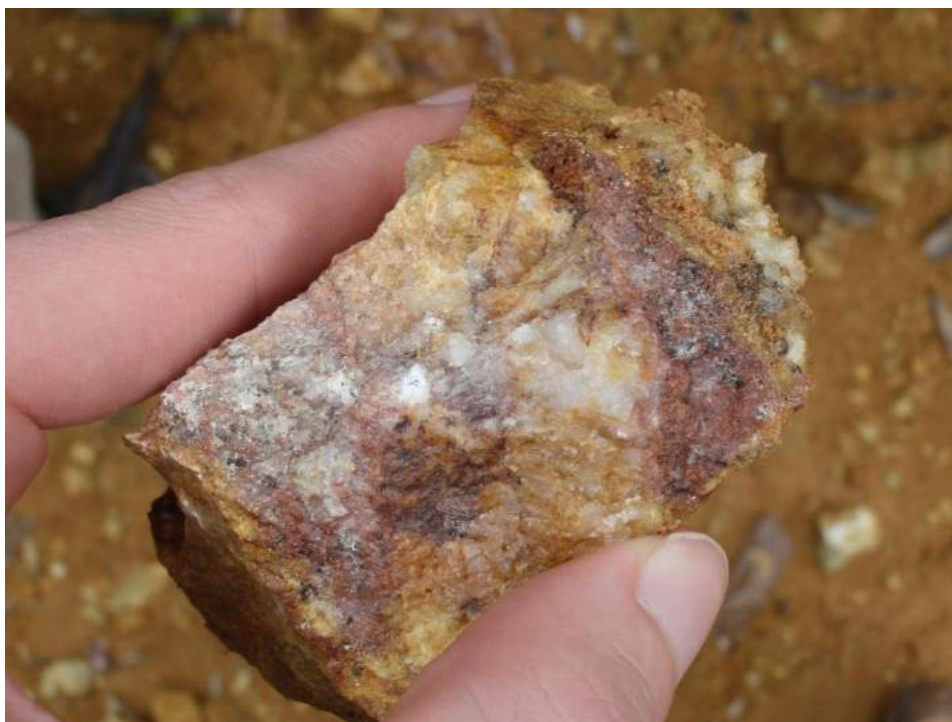
Figure 9.2 Oxidised quartz-pyrite veining proximal to the Bukit Tujoh intrusive contact, Harimau Prospect
