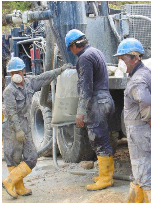
Figure 12.7 Collecting wet sample off cyclone
